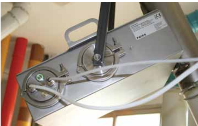
Mounted directly in production, the ProFoss measures the flour as it flows through pipes at up to 25 metres a second
