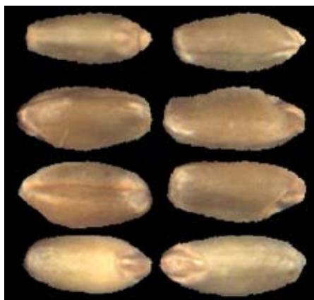
Figure 2. Example of images from a Cervitec™ 1642 showing Australian durum wheat. An ANN calibration predicted the six first kernels as vitreous (hard kernels that form good semolina for pasta making), the next one as non-vitreous (opaque kernel) and the last one bleached (the surface makes it hard to see through the kernel).
