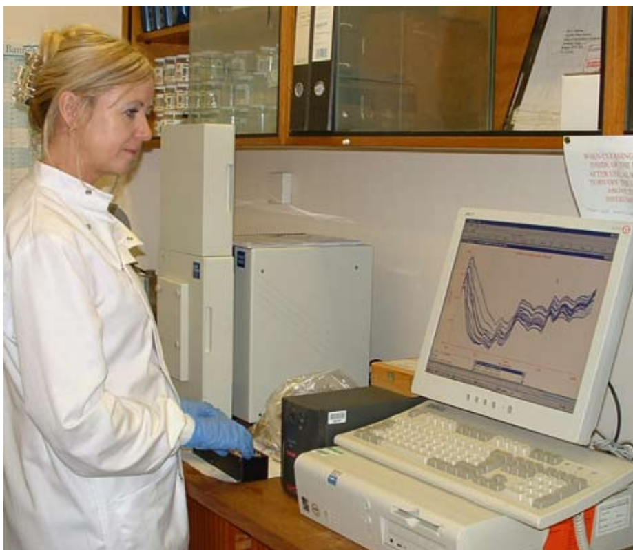
Vis-NIR spectrometer for assessing quality of raw materials and substrate
